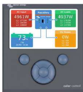
Color Control GX, showing a PV application
